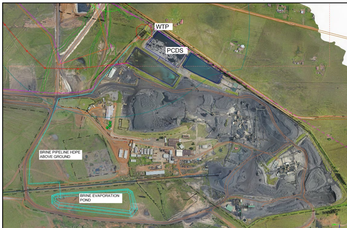
Figure 2-5: Brine PCD & pipeline layout.
