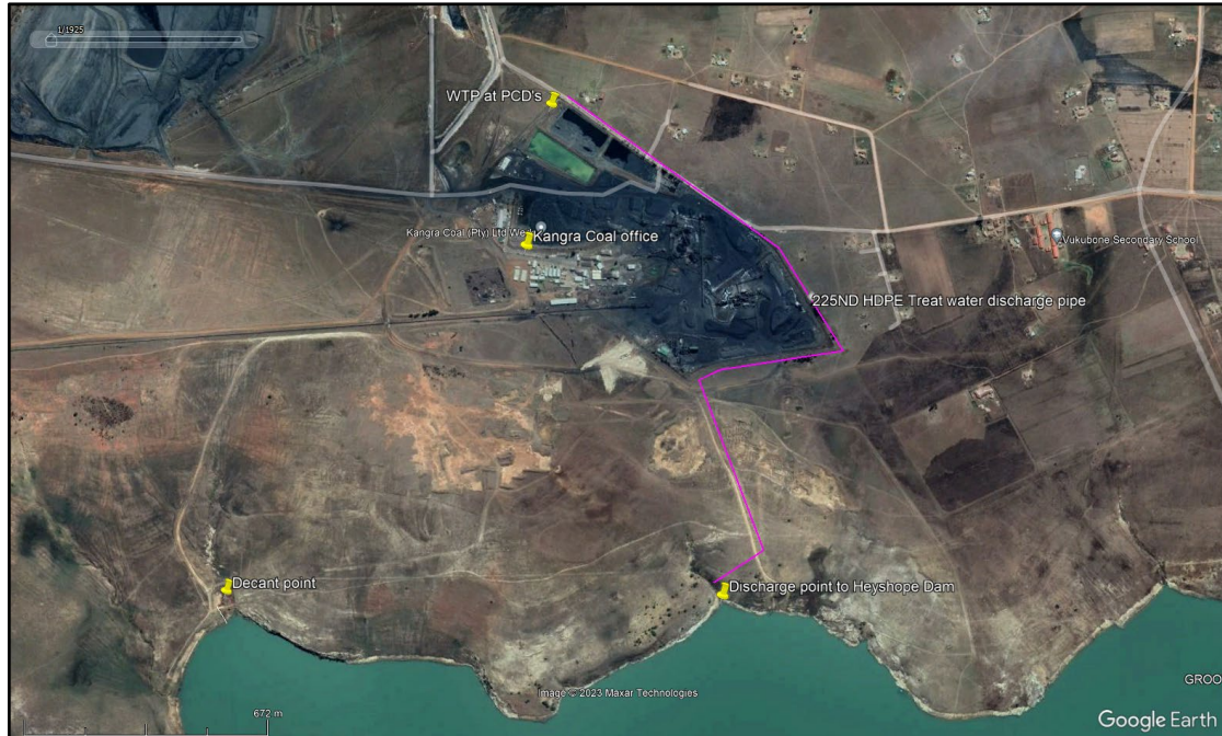
Figure 2-6: WWTP discharge pipeline.
