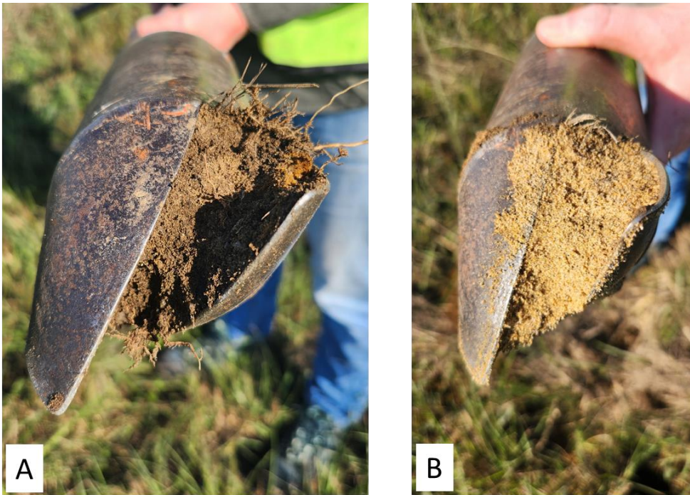
Figure 15: Soils identified in the infrastructure site including (A) the Witbank soil which includes deposited material on top of (B) the original estuarine soils
