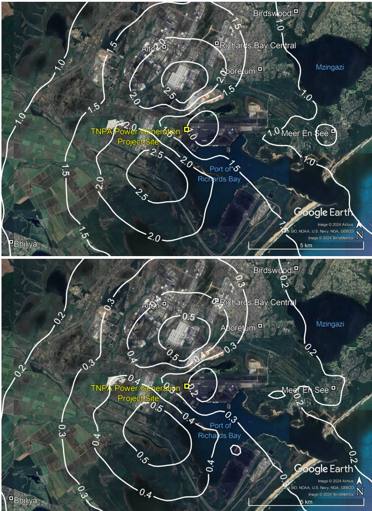
Figure 6-14: Predicted 99 th percentile 1-hour NO 2 concentrations in µg/m 3 resulting from emissions from the TNPA 22 MW Duel Fuel Generator for Scenario 1 where diesel fuel is used (top) and for Scenario 2 where LNG fuel is used (bottom)
