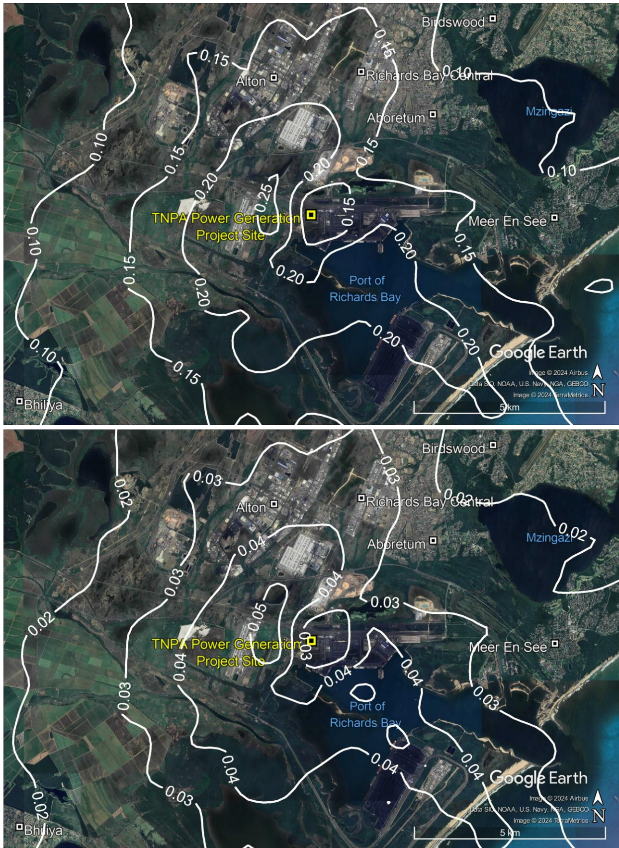
Figure 6-16: Predicted 99 th percentile 24-hour PM 10 concentrations in µg/m 3 resulting from emissions from the TNPA 22 MW Duel Fuel Generator for Scenario 1 where diesel fuel is used (top) and for Scenario 2 where LNG fuel is used (bottom)
