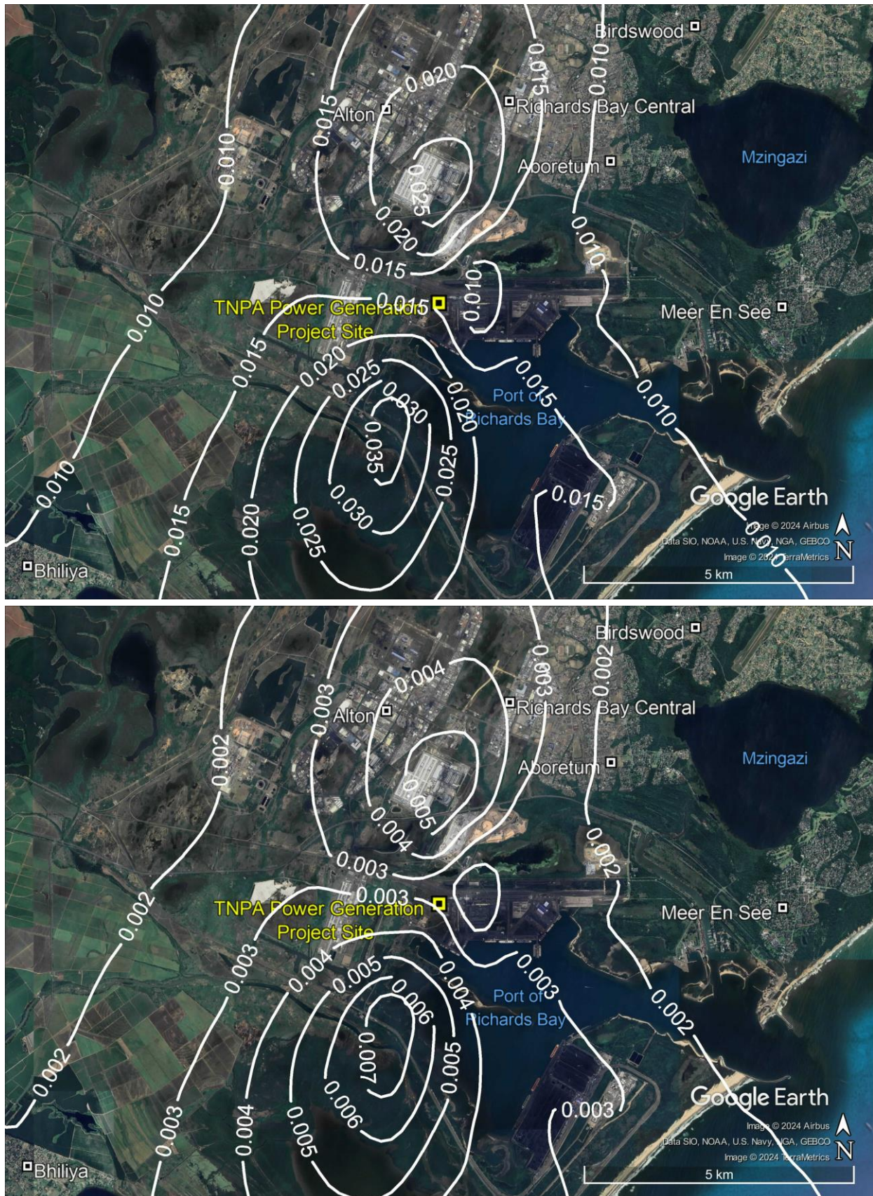
Figure 6-15: Predicted annual average PM 10 concentrations in µg/m 3 resulting from emissions from the TNPA 22 MW Duel Fuel Generator for Scenario 1 where diesel fuel is used (top) and for Scenario 2 where LNG fuel is used (bottom)
