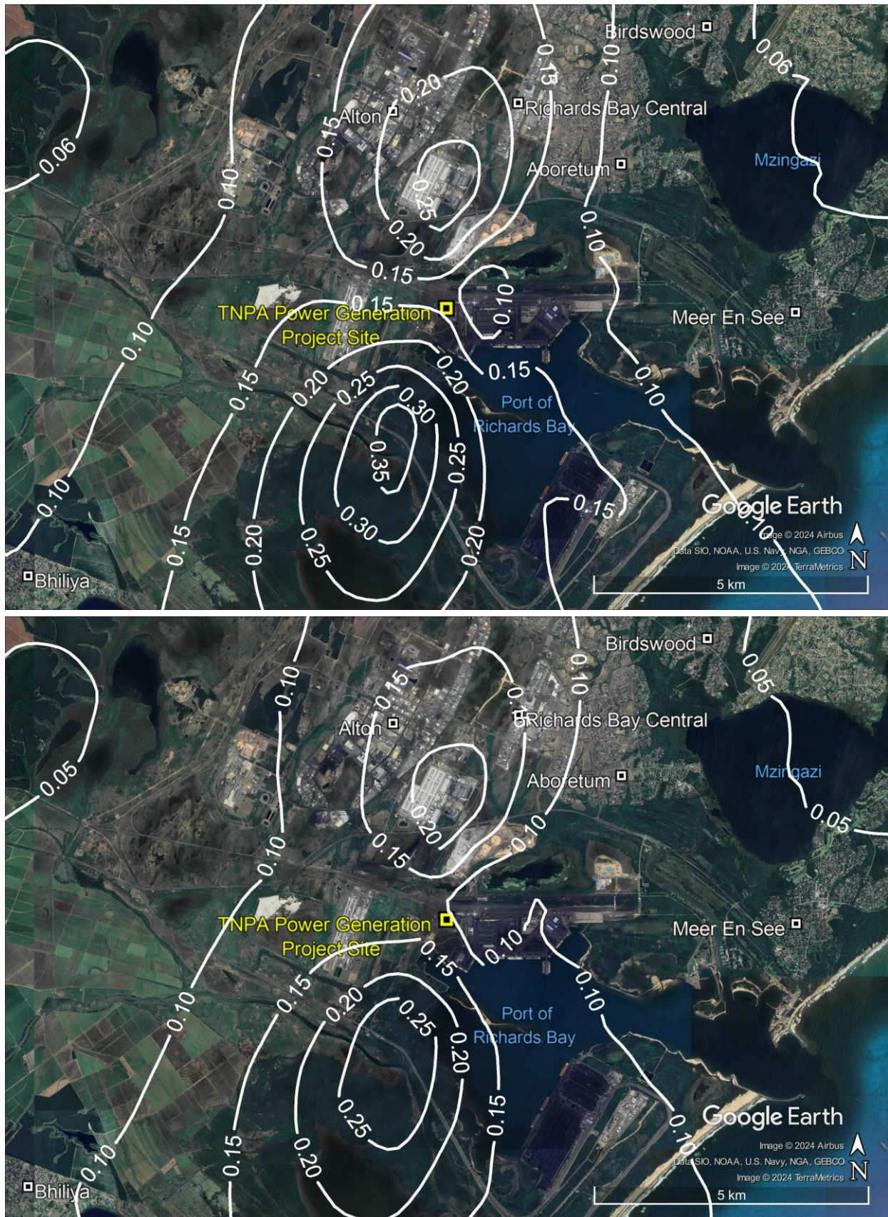
Figure 6-10: Predicted annual average SO 2 concentrations in µg/m 3 resulting from emissions from the TNPA 22 MW Duel Fuel Generator for Scenario 1 where diesel fuel is used (top) and for Scenario 2 where LNG fuel is used (bottom)
