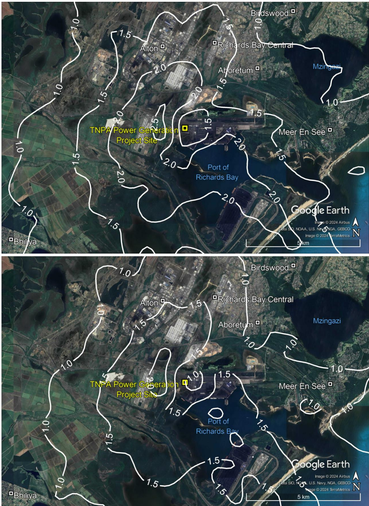
Figure 6-11: Predicted 99 th percentile 24-hour SO 2 concentrations in µg/m 3 resulting from emissions from the TNPA 22 MW Duel Fuel Generator for Scenario 1 where diesel fuel is used (top) and for Scenario 2 where LNG fuel is used (bottom)
