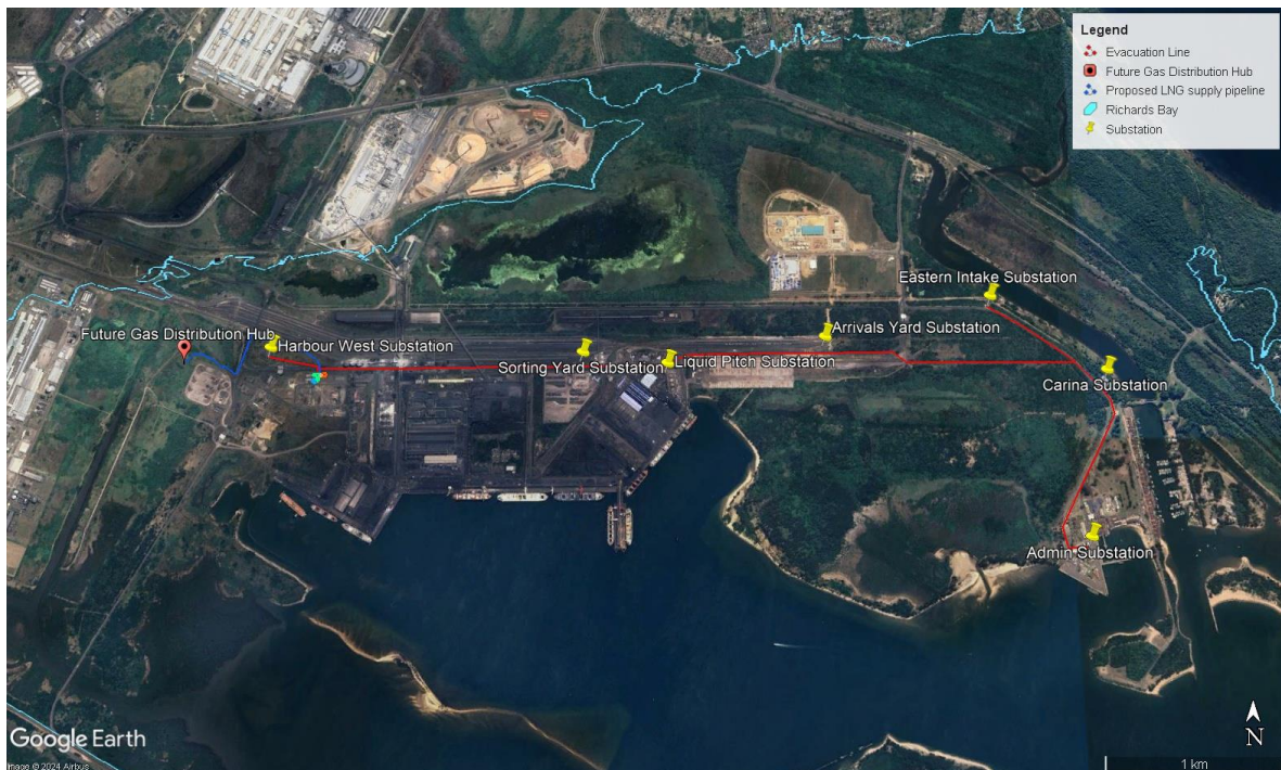
Figure 1. Proposed layout for the TNPA 22MW Dual Fuel Generator Project, Richards Bay. The Estuarine Functional Zone (EFZ) of the Richards Bay estuary is shown in light blue.
