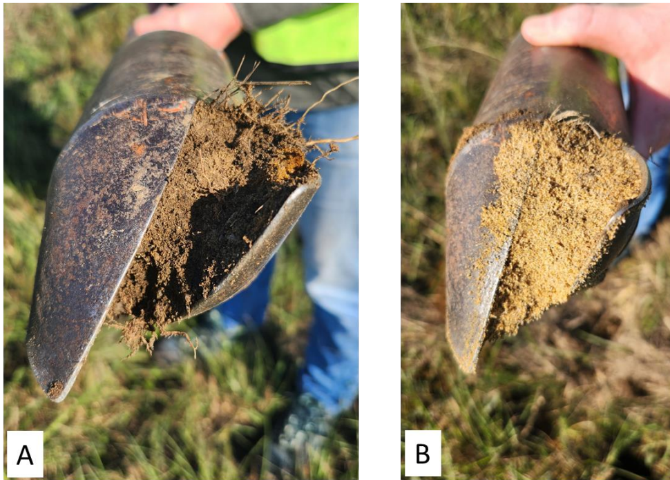
Figure 11: Soils identified in the infrastructure site including (A) the Witbank soil which includes deposited material on top of (B) the original estuarine soils
