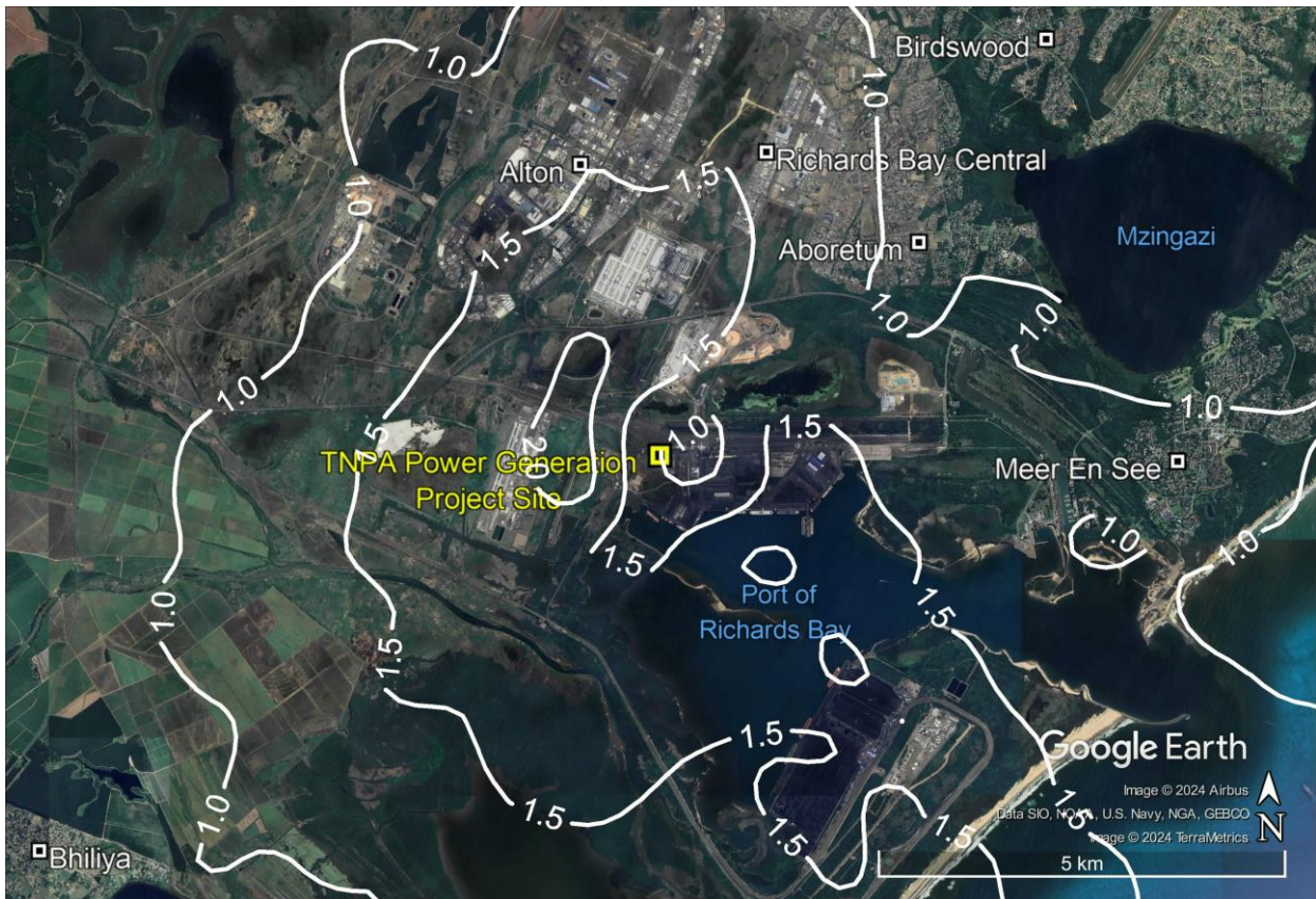
Figure 6-11: Predicted 99 th percentile 24-hour SO 2 concentrations in \mu\text{g}/\text{m}^3 resulting from emissions from the TNPA 22 MW Duel Fuel Generator for Scenario 1 where diesel fuel is used (top) and for Scenario 2 where LNG (in natural gas form) fuel is used (bottom)
