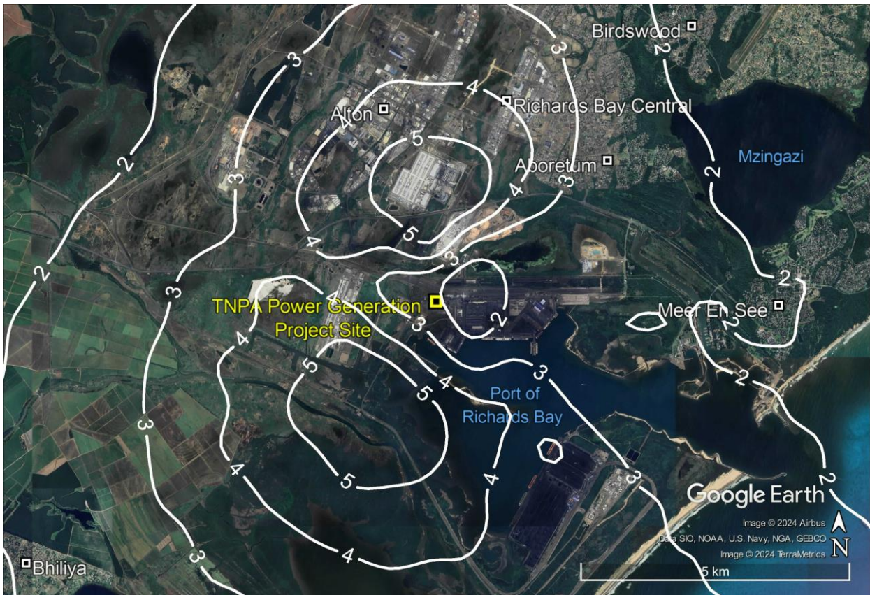
Figure 6-12: Predicted 99 th percentile 1-hour SO 2 concentrations in µg/m 3 resulting from emissions from the TNPA 22 MW Duel Fuel Generator for Scenario 1 where diesel fuel is used (top) and for Scenario 2 where LNG (in natural gas form) fuel is used (bottom)
