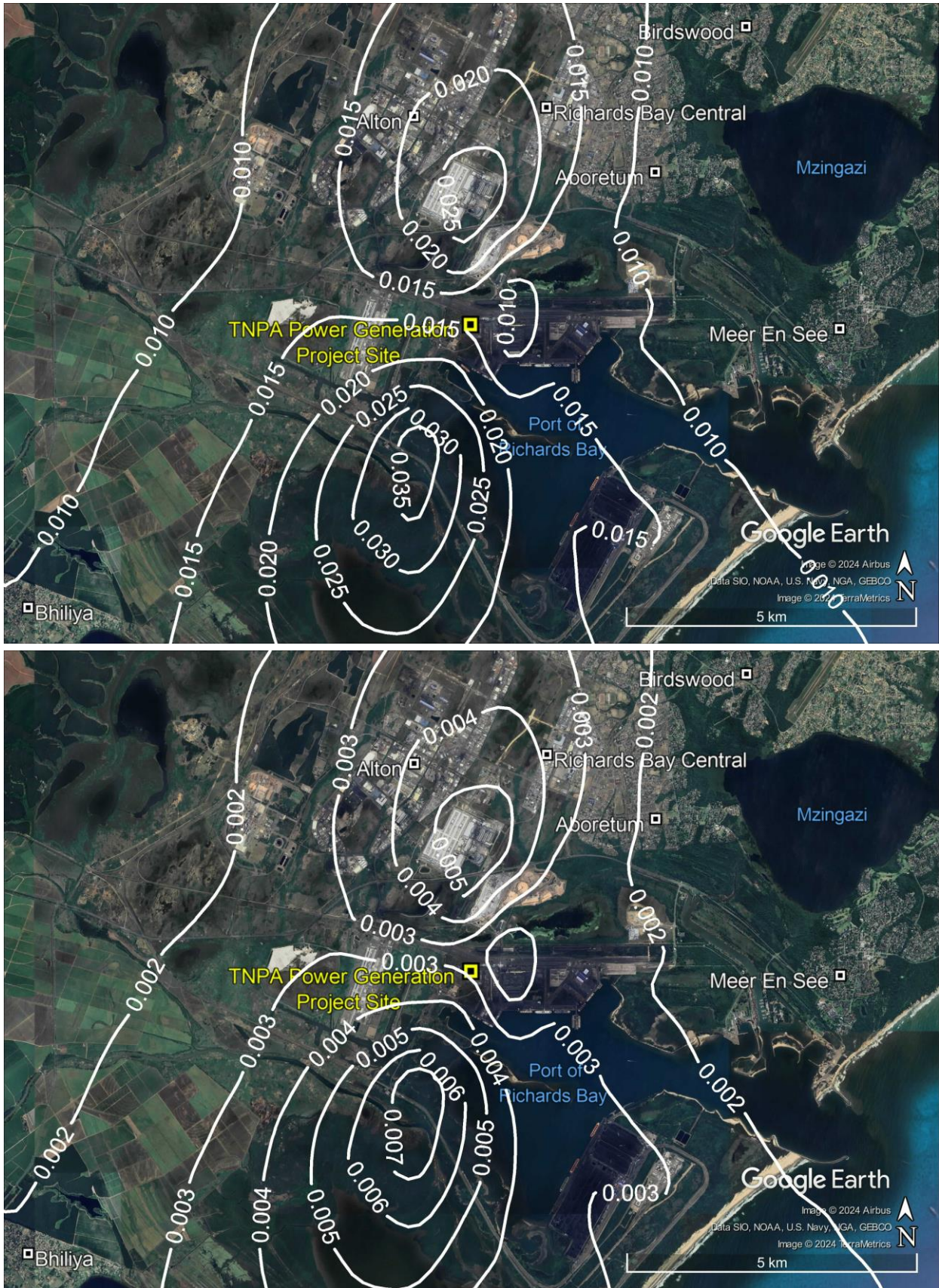
Figure 6-15: Predicted annual average PM 10 concentrations in µg/m 3 resulting from emissions from the TNPA 22 MW Duel Fuel Generator for Scenario 1 where diesel fuel is used (top) and for Scenario 2 where LNG (in natural gas form) fuel is used (bottom)
