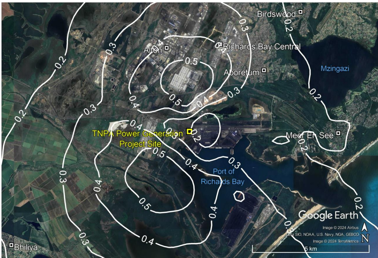
Figure 6-14: Predicted 99 th percentile 1-hour NO 2 concentrations in µg/m 3 resulting from emissions from the TNPA 22 MW Duel Fuel Generator for Scenario 1 where diesel fuel is used (top) and for Scenario 2 where LNG (in natural gas form) fuel is used (bottom)
