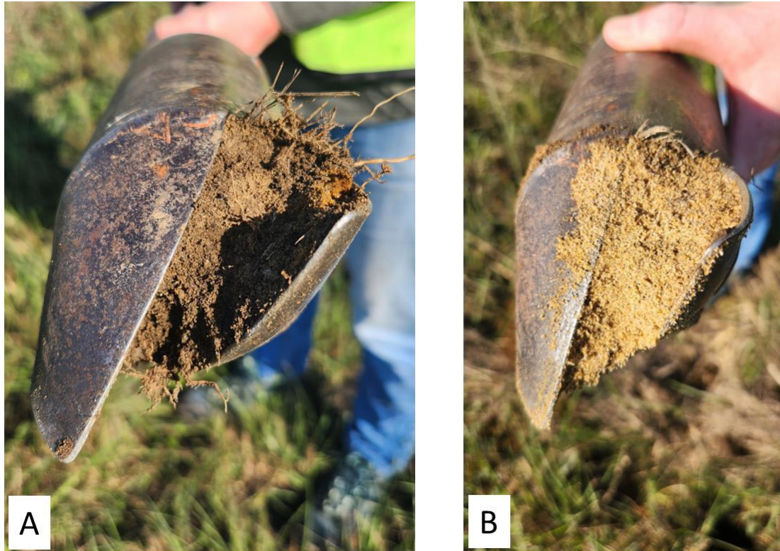
Figure 7-6: Soils identified in the infrastructure site including (A) the Witbank soil which includes deposited material on top of (B) the original estuarine soils. Pictures were taken during the site visit on 8 th of May 2024.
