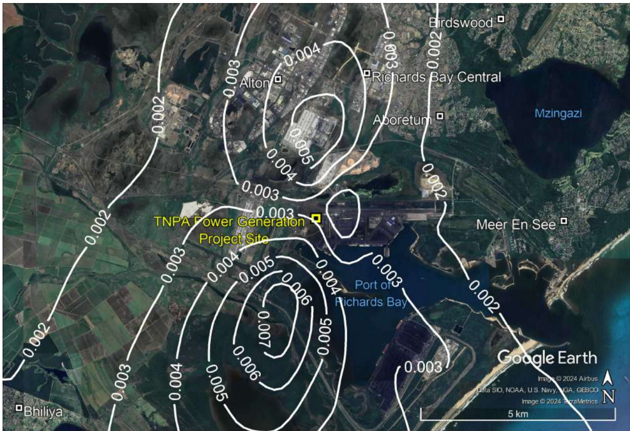
Figure 6-15: Predicted annual average PM 10 concentrations in µg/m 3 resulting from emissions from the TNPA 22 MW Duel Fuel Generator for Scenario 1 where diesel fuel is used (top) and for Scenario 2 where LNG (in natural gas form) fuel is used (bottom)
