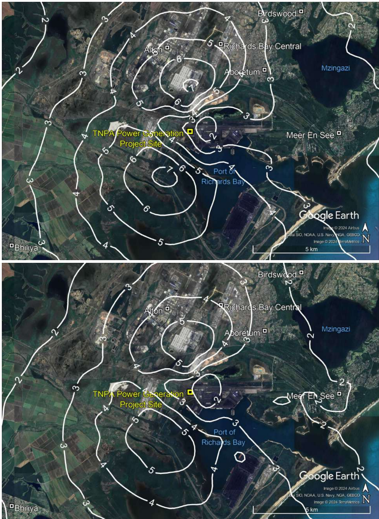
Figure 6-12: Predicted 99 th percentile 1-hour SO 2 concentrations in µg/m 3 resulting from emissions from the TNPA 22 MW Duel Fuel Generator for Scenario 1 where diesel fuel is used (top) and for Scenario 2 where LNG (in natural gas form) fuel is used (bottom)
