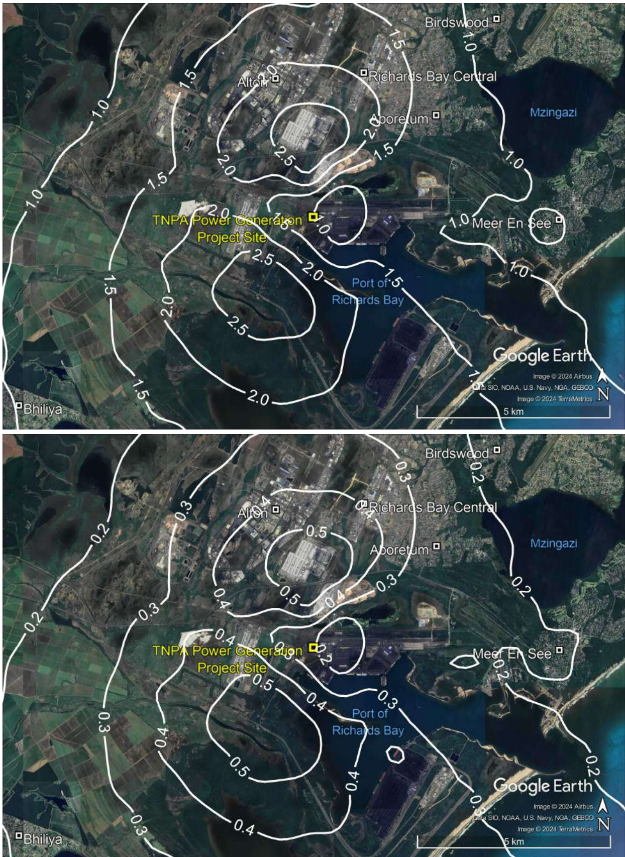
Figure 6-14: Predicted 99 th percentile 1-hour NO 2 concentrations in µg/m 3 resulting from emissions from the TNPA 22 MW Duel Fuel Generator for Scenario 1 where diesel fuel is used (top) and for Scenario 2 where LNG (in natural gas form) fuel is used (bottom)
