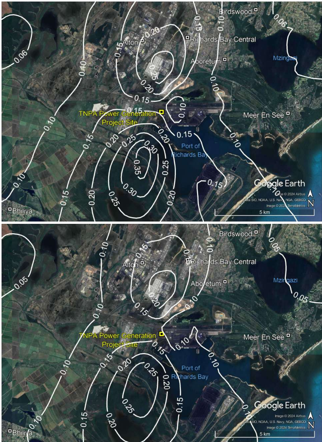
Figure 6-10: Predicted annual average SO 2 concentrations in µg/m 3 resulting from emissions from the TNPA 22 MW Duel Fuel Generator for Scenario 1 where diesel fuel is used (top) and for Scenario 2 where LNG (in natural gas form) fuel is used (bottom)
