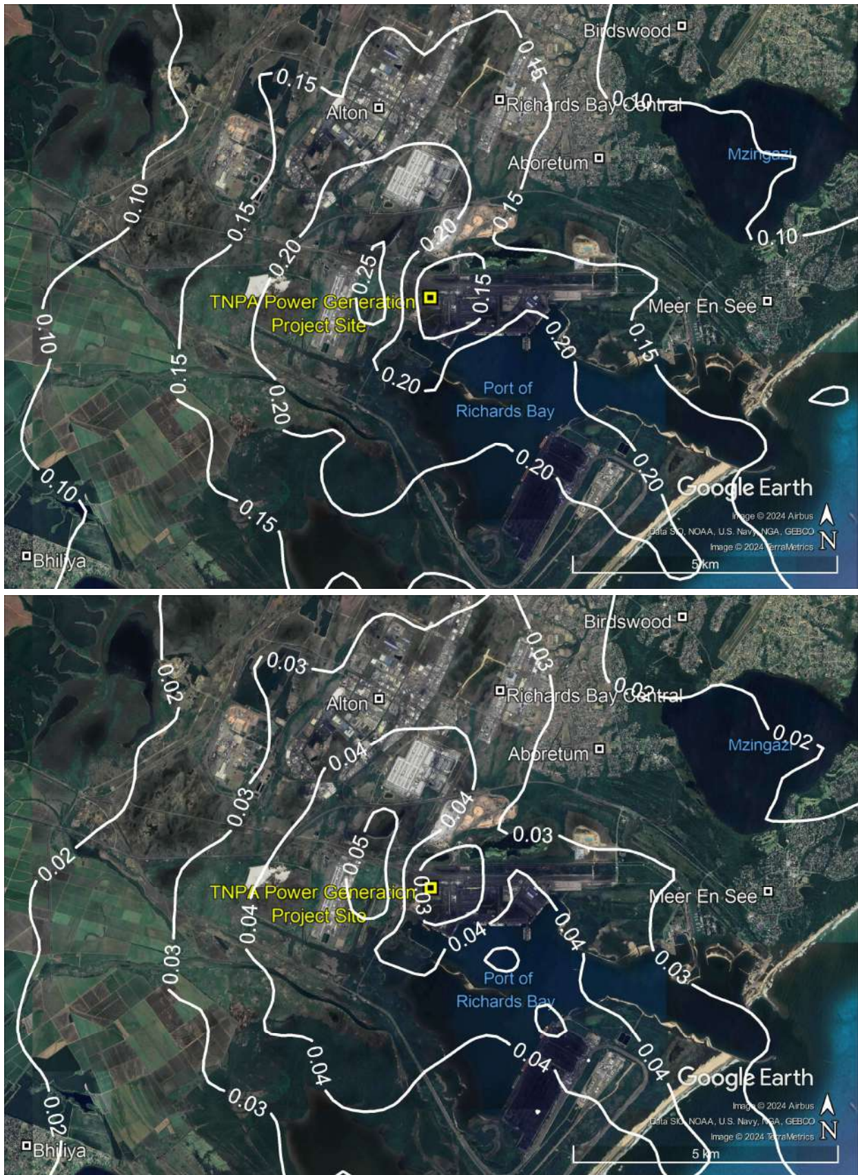
Figure 6-16: Predicted 99 th percentile 24-hour PM 10 concentrations in µg/m 3 resulting from emissions from the TNPA 22 MW Duel Fuel Generator for Scenario 1 where diesel fuel is used (top) and for Scenario 2 where LNG (in natural gas form) fuel is used (bottom)
