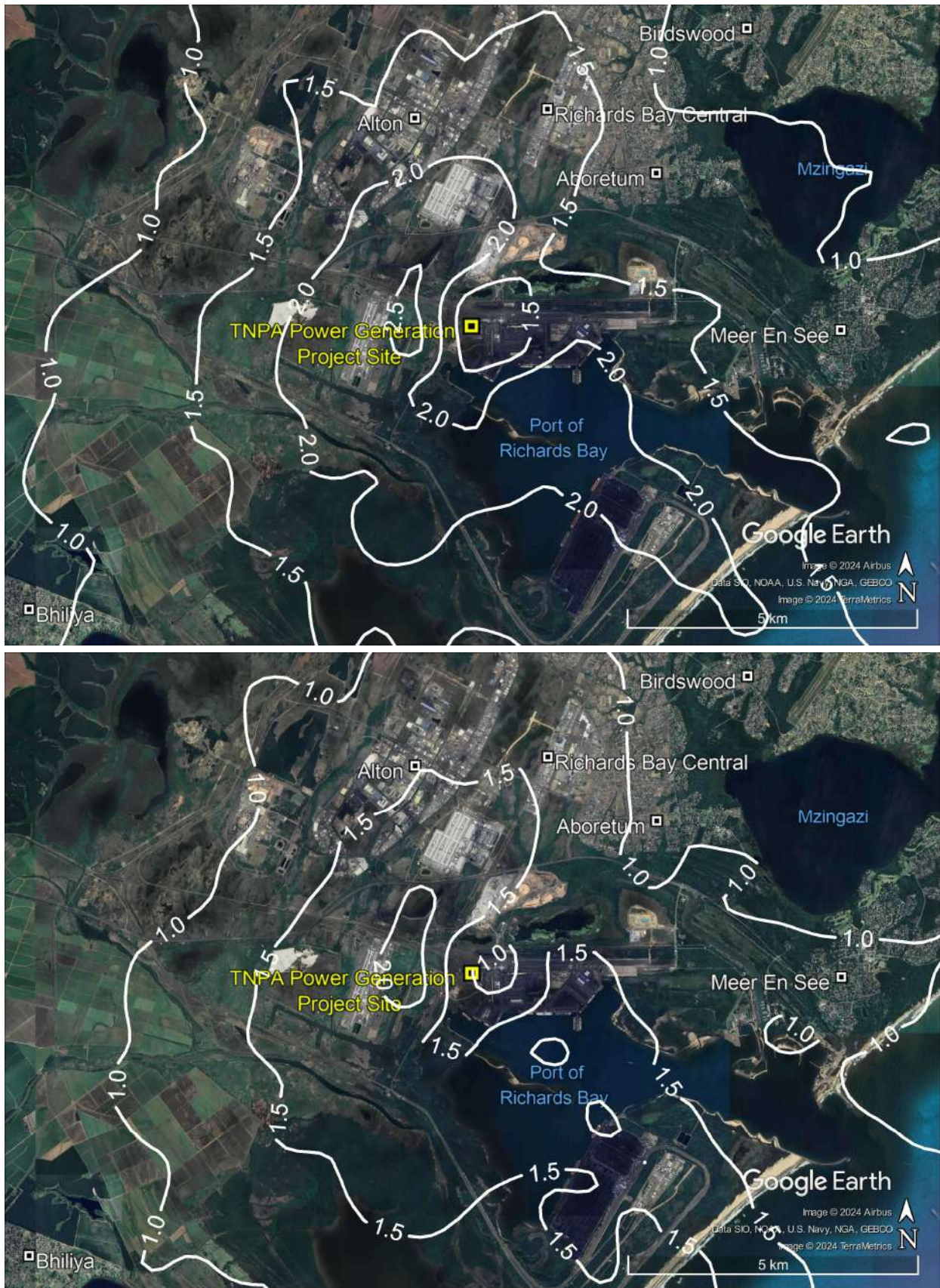
Figure 6-11: Predicted 99 th percentile 24-hour SO 2 concentrations in µg/m 3 resulting from emissions from the TNPA 22 MW Duel Fuel Generator for Scenario 1 where diesel fuel is used (top) and for Scenario 2 where LNG (in natural gas form) fuel is used (bottom)
