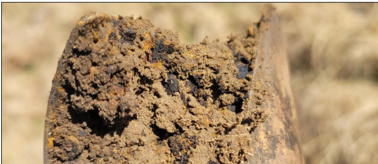
Figure 8-2: Shows the Plinthic concretions in the lower soil profile of the Tukulu soil.
