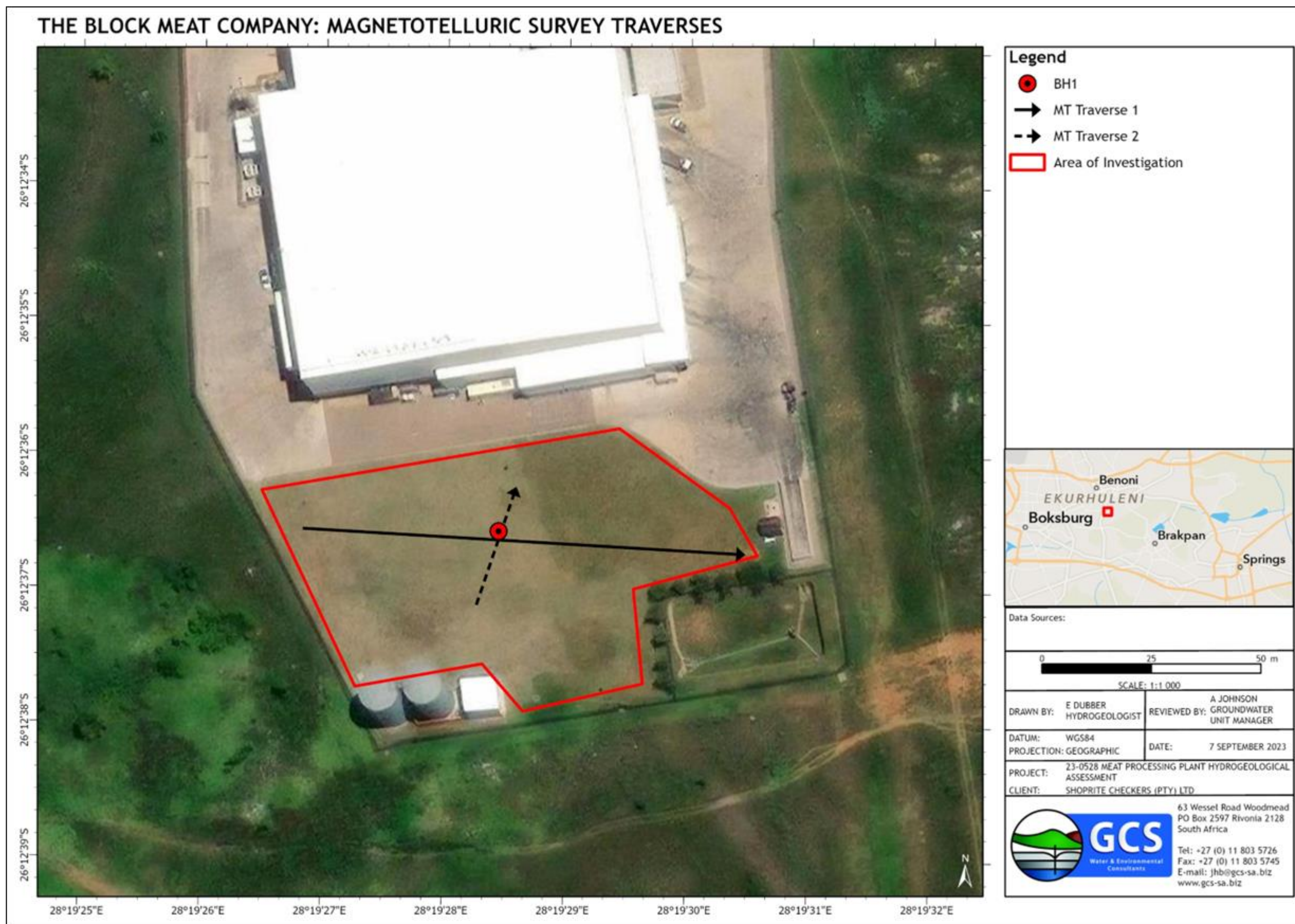
Figure 4.3: MT survey traverses and borehole BH1 location.
